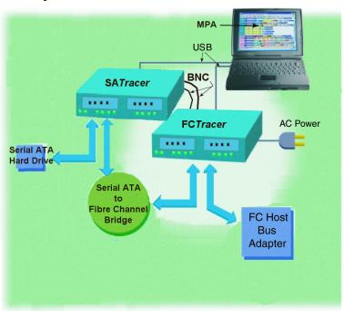
A hypothetical test setup: a Serial ATA hard drive connected to a bridge, and the bridge, in turn, is connected to a Fibre Channel HBA. Two *cascaded* analyzers are placed on the links and administered by a laptop running MPA. In this setup, MPA will be able to instruct both analyzers to simultaneously record, give the recordings a common timestamp, and afterwards analyze the two traces side-by-side.
